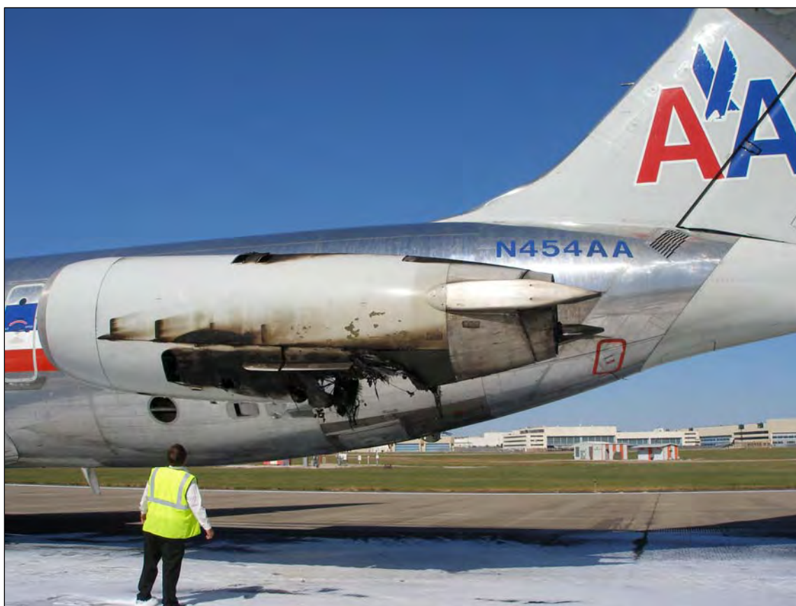
Figure 1. Photograph of the left side of the airplane after fire-extinguishing efforts were completed.
